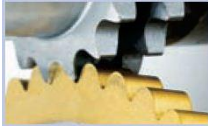
Figure N°2- Rolling operation of a chain sprocket
